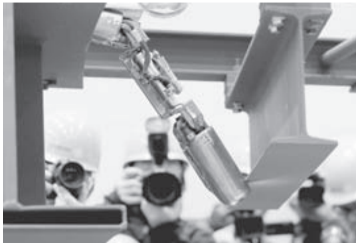
In this Thursday, Feb. 5, 2015 file photo, a remote-controlled robot that looks like an enlarged fiberscope crawls down into the mock-up of a primary containment chamber of Fukushima Dai-ichi nuclear plant, during a demonstration for the media at a government facility in Hitachi, Ibaraki Prefecture, northeast of Tokyo.
